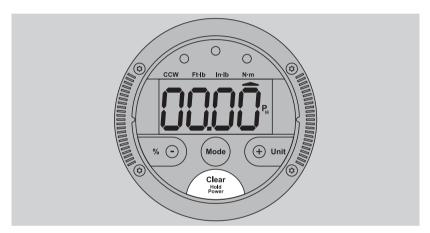
If the batteries' or rechargeable batteries' state of charge is too low, the DPG cannot be switched on, or immediately switches off again.
