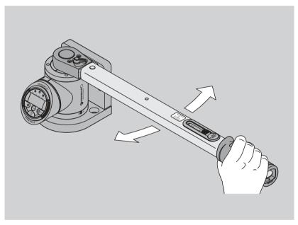
If you have discovered deviations from the nominal values, adjust and calibrate the torque wrench as described in the respective operating instructions, and then test the torque wrench again.
